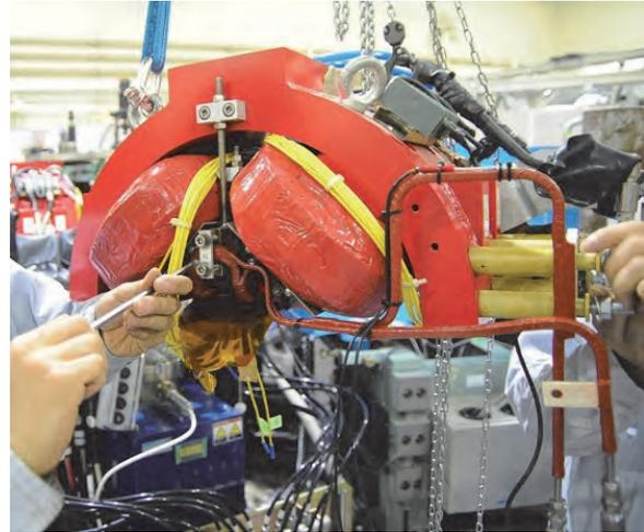
Fig. 2. Replacing sextupole coil for multipole magnets.
